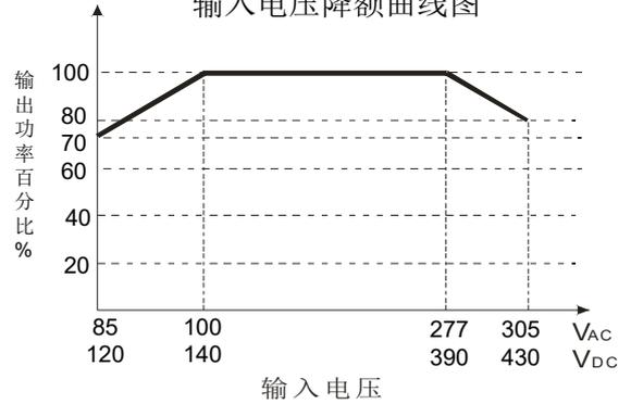
注:①对于输入电压为85~100Vac/277~305Vac/122~140Vdc/390~430Vdc,需在温度降额的基础上进行电压降额;
